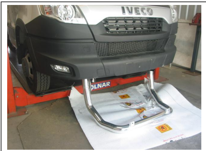
Figure 3: Protection bar fitment, on soft covering with rear bolts installed.
