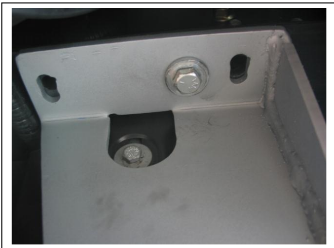
Figure 1: Passengers side shown. Use M10 x 35 bolt, flat washer and spring washer only
